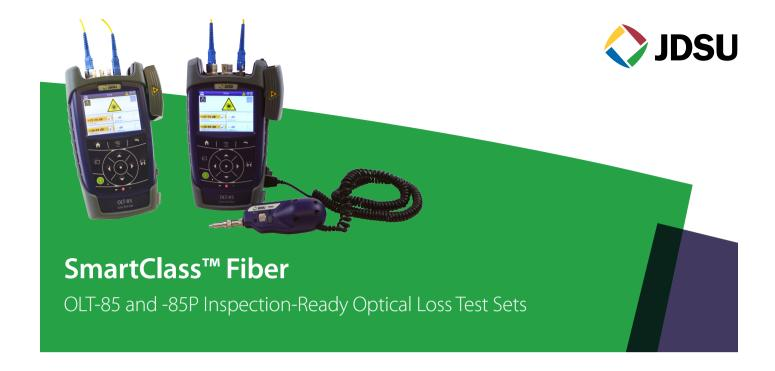
The SmartClass Fiber OLT-85 and -85P combine a fiber inspection microscope, optical power meter (OPM), and optical light source (OLS) in one versatile test instrument. The compact instrument provides the essential fiber tests—inspection, power, insertion loss, and continuity—for multimode and single-mode networks.
